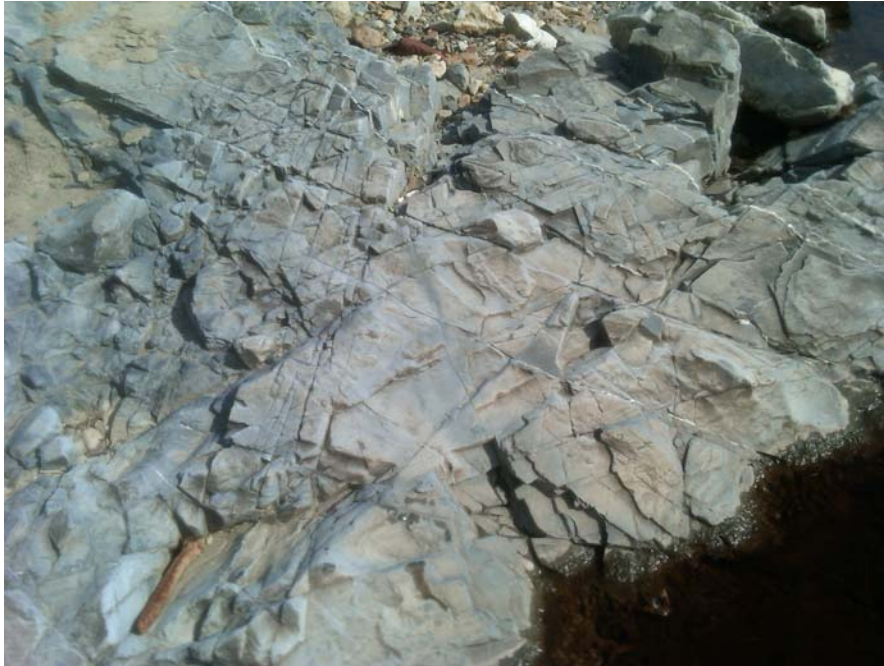
Photo 5: Eastward and downward view of gray limestone and dolostone of the Vintage Formation below the transitional beds at outcrop along Codorus Creek. Shows various joint sets and closely spaced jointing on the left. RR spike shows scale.
